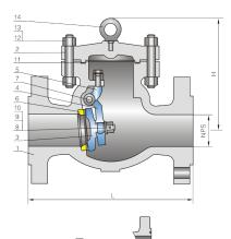
Notes: 1). Cast steel disc for NPS 4" and above.
